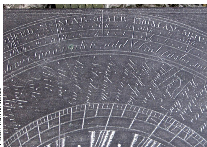
Fig. 13. Part of the EoT ring on a multiple-gnomon slate dial by Richard Melville. This Sussex dial, from relatively late in Melville's career, has the correct value of 4 mins for May 20.
