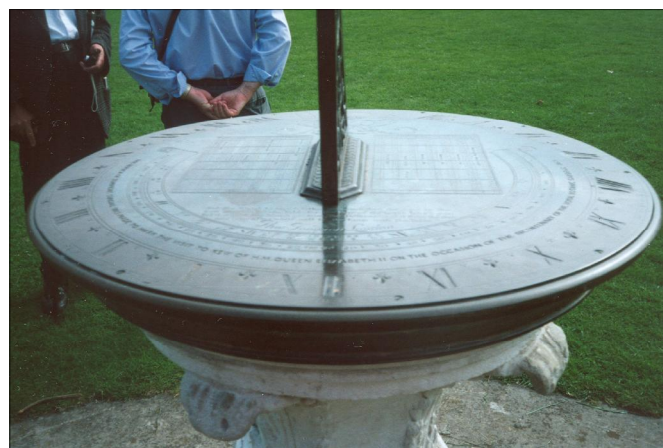
Above: the 1952 replica of the Hampton Court Tompion dial, made to commemorate a visit of the Queen. Note the large EoT table and the azimuth scale centred on the vertical back edge of the gnomon.
