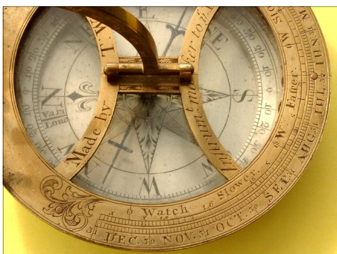
Fig. 5. A mechanical equinoctial dial by Thomas Wright.
