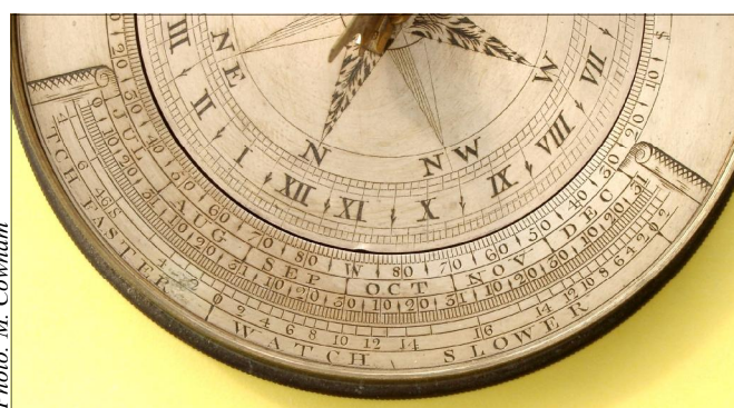
Fig. 6. A magnetic compass dial by Fraser.
