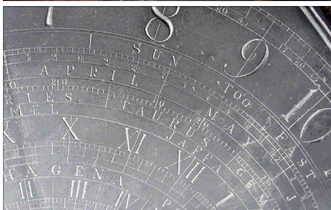
Fig. 11. An 1825 slate dial by Samuel Eason:(top) prior to its recent restoration;(bottom)part of EoT scale in degrees of solar longitude. Courtesy of David Harber Sundials.
